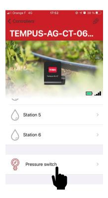
Select the new icon "Pressure Switch" on your device which is displayed at the bottom of the screen.
