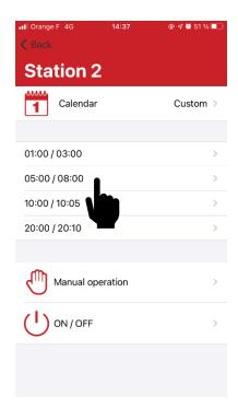
i Each station is independent and can get a different periodicity or irrigation cycle regarding the others. Each station can get up to maximum 4 watering windows.
