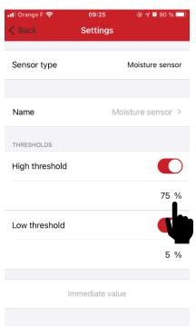
In the settings area, you can define the high and low thresholds for which you want to receive an alert.
