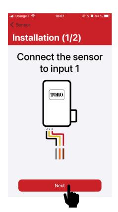
Follow the wiring scheme of the type EC5-SOIL moisture sensor displayed on your app in order to connect it and then select "Next".
