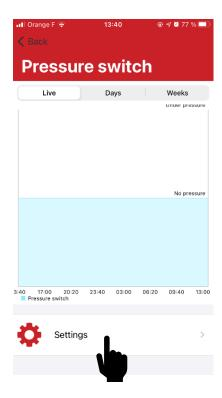
You can visualize if the pressure has been reached or not by checking data per live (last 24 hours), days, weeks. If value = 1, the pressure tuned has been reached. If value = 0, the pressure tuned has not been reached.
